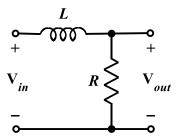
a. Determine an expression for the voltage transfer function,  $\mathbf{V}_{out}/\mathbf{V}_{in}$ . Also, determine expressions for the magnitude and the phase angle of that transfer function.
